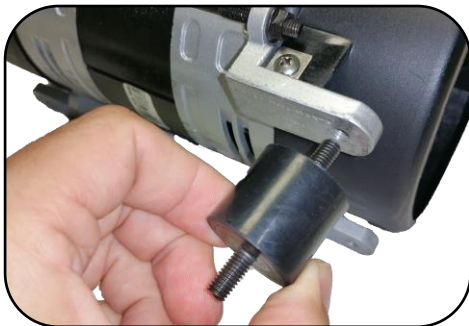
Install Shock Absorbing Mounts (Prepare location the Air Compressor will be mounted)
