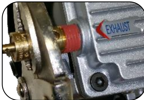
Install Pressure Release Valve (Exhaust Port opposite of desired Air Fitting location)
